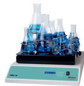
HSM 10 including platform for Erlenmeyer flasks, with a set of 6 different clamps
