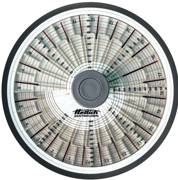
View into the centrifuging chamber showing rotor 2076 with lid as evaluation disc
