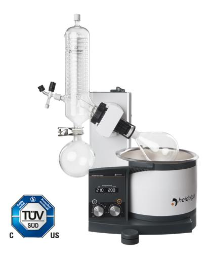
The Hei-VAP Value Digital rotary evaporators with hand lift are optimally suited for all standard applications with a digital display for set and actual heating bath temperature.
