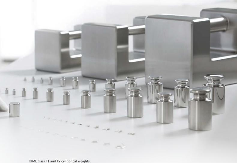
OIML class F1 and F2 cylindrical weights with a lug are made of a special stainless steel that has a density of 7,950 kg/m³, and their tolerances comply with OIML R111-1. The weights are delivered in a wooden case suitable for transportation by a pallet mover.
