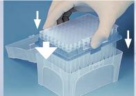
Insert the filled tip-tray perpendicularly from above into the previously sterilized TipBox until it locks into place.
