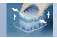
Press the long sides of the transfer aid together, and continue pressing them together while withdrawing the tip-tray.
