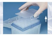
Remove the transfer aid from the mounting plate. Finished – all without tip contact!
