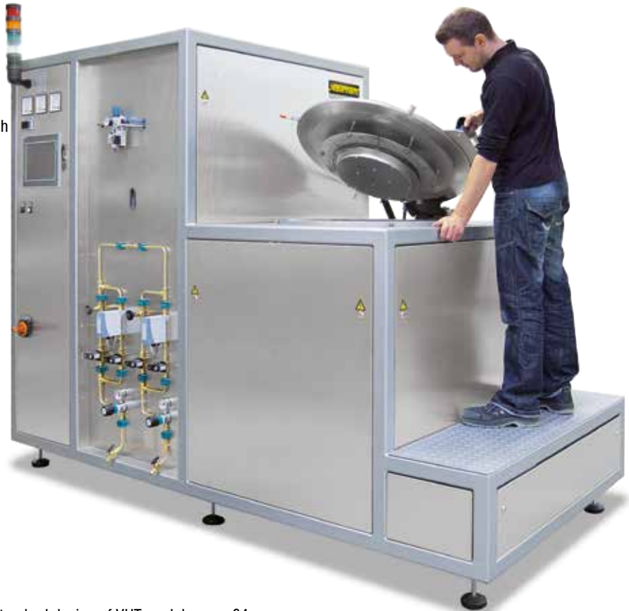
Retort furnace SVHT 9/24-W with tungsten heating
