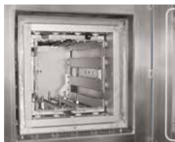
Molybdenum or tungsten heating chamber
