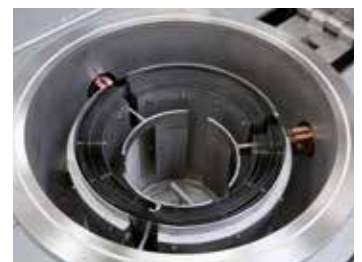
Cylindrical retort with tungsten heating
