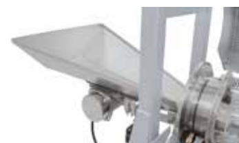
Vibrating channel on the rotary tube for convenient material feeding
