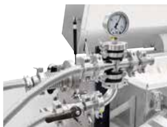
Connection set for vacuum operation
